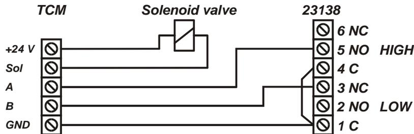
The TCM port should be set to control the appropriate PC tank in relation to the physical tank. Correct TankType, TCMAAddress and TCMPort should be set using with WinDB Manager.
