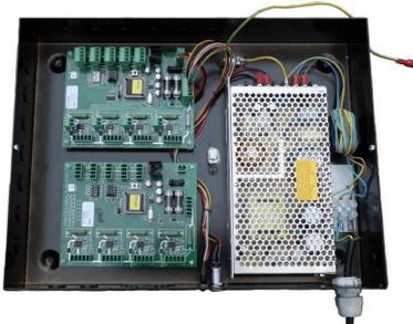
Fasten the short plastic distances so the new card can be placed closest to the bottom like in the picture.
