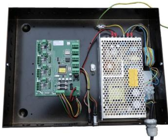
Make sure that the TCM is disconnected from the mains power supply and the ORILINK® network before any work is started. Use a voltmeter to make sure that there is no power.
