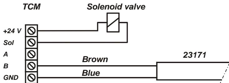
The TCM port should be set to control the appropriate PC tank in relation to the physical tank. Correct TankType, TCMAAddress and TCMPort should be set using with WinDB Manager.
