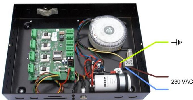
The power supply should be connected to mains 230VAC in a proper way following valid rules.
