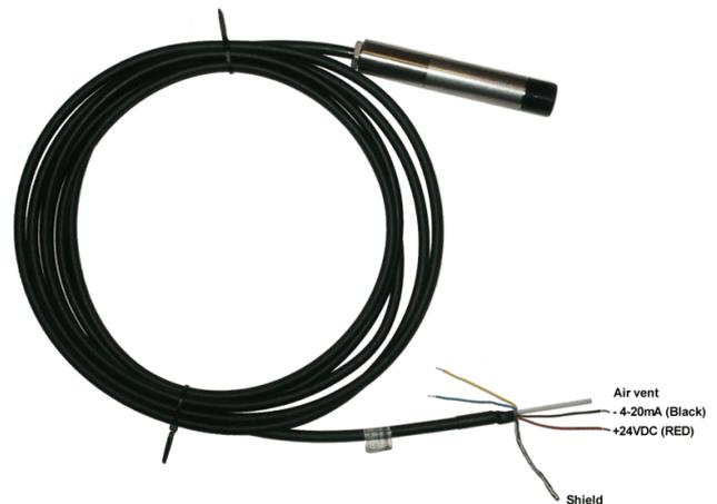
**OBSERVE!** It is important that the transparent tube is not blocked and that the humidity protection filter is used. A blocked tube will cause measuring failure. Not using the humidity protection could cause sensor malfunction due to corrosion caused by condensed water.
