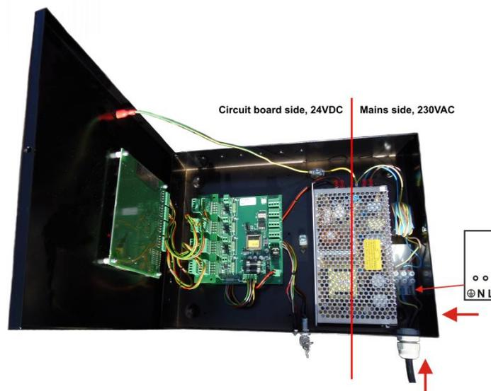
The TSM is equipped with a switched power supply of 150W that can be set for 110VAC/60Hz or 230VAC/50Hz by the internal switch shown by the yellow sticker.
