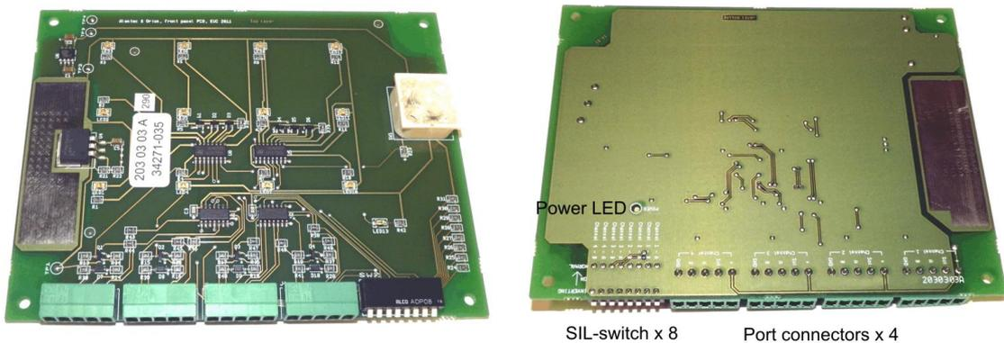
The indicator board is powered by the Port 1 inter connection cable. If the board has power (24VDC) the power led (see picture) will be lit.
