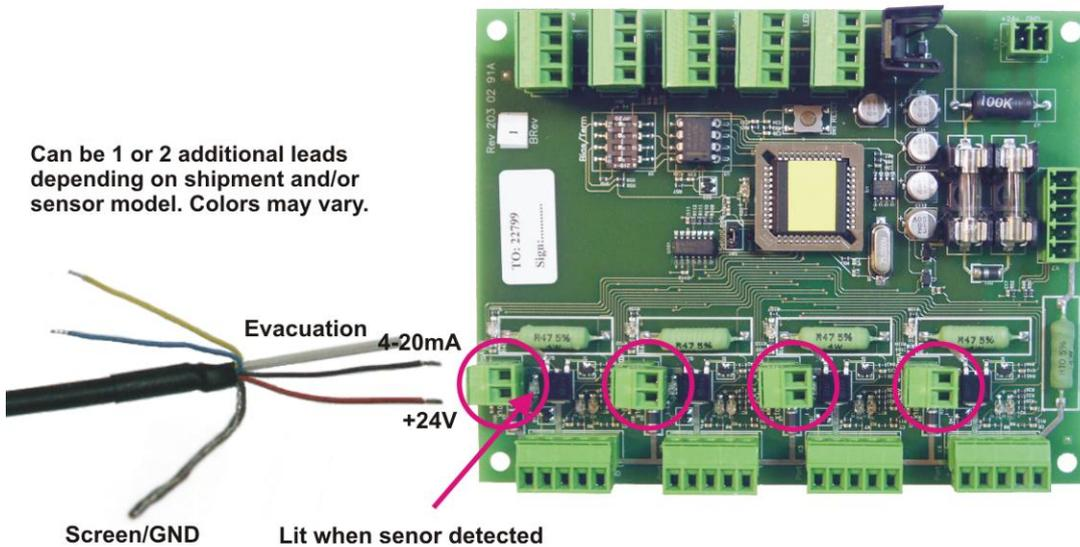
Correct TankType, TSMAddress and TSMPort should be set using with WinDB Manager
