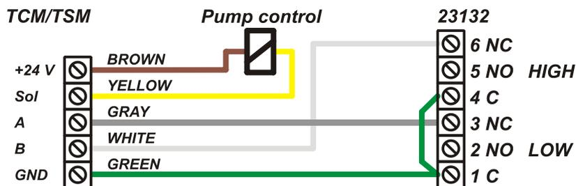
The TSM port should be set to control the appropriate PC tank in relation to the physical tank. Correct TankType, TSMAddress and TSMPort should be set using with WinDB Manager
