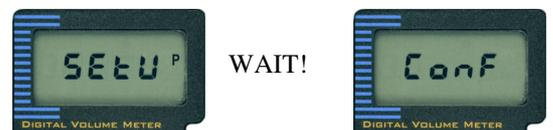
To get back to normal operation mode wait a short time or press <RESET> button. When the display looks like this it is done.
