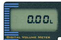
Press <RESET> and the meter will do a re-set and show all the segments of the LCD for a short while.
