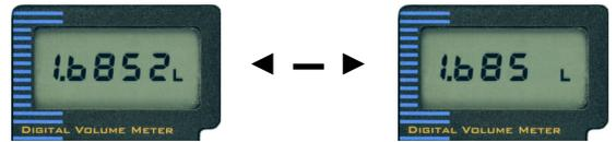
When the last figure is blinking and <SELECT> is pressed the display will change to show the calculated calibration factor. If <RESET> is pressed the new calibration is cancelled.
