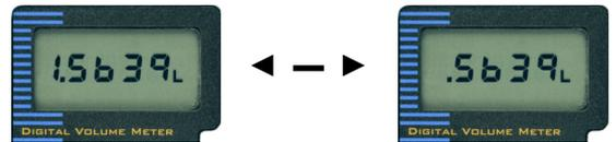
In this example we received 1.6852 L so we move to second figure with <SELECT> and change it from 5 to 6 with <RESET> move to third figure and change it from 6 to 8 and so on.
