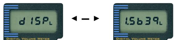
Then press <SELECT> and the display will move on to received volume input. The first figure will “blink” to show that it is changeable. Press <RESET> to change the value press <SELECT> to change to the next figure.
