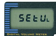
Scroll through the different units using the <RESET> button. L, G, P, Q, L,..... . When the wanted unit is shown release all buttons and wait. The will save and go back to “ConF” after a short time.
