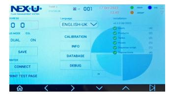
2. Or, you can go to the configuration menu and only one code is required. The code is CAL
