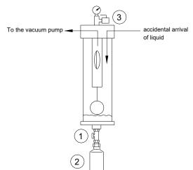
Once the pot is empty, it is possible that the level sensor (mechanical closure valve) might remain in the closed position. To release it, simply open valve ③ and close it again.
