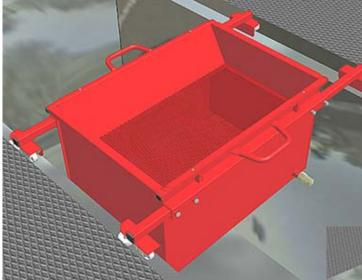
When the unit is full (**level with the underside of the filter mesh**) it can be emptied from the outlet port at the bottom of the tank. This is supplied with a 3/4"bsp quick release coupling to enable simple hose connection to a suitable waste oil pump (mounted either in the pit or in close proximity to the pit) to pump the oil to a designated bulk storage vessel.
