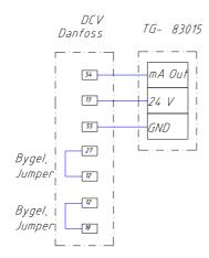
Application with start/stop via external NO (normally open) contact, e.g. 88400.
