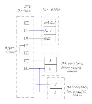
Application with integration of Alentec & Orion AB control equipment for start/stop.
